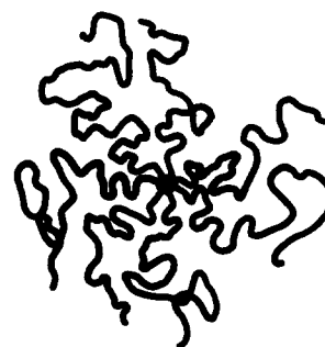
Figure 1 Schematic representation of estimated micelle structure formed in CBC
